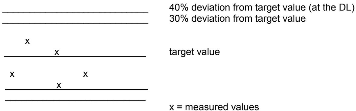
**Fig. 1: example picture of a control chart**
