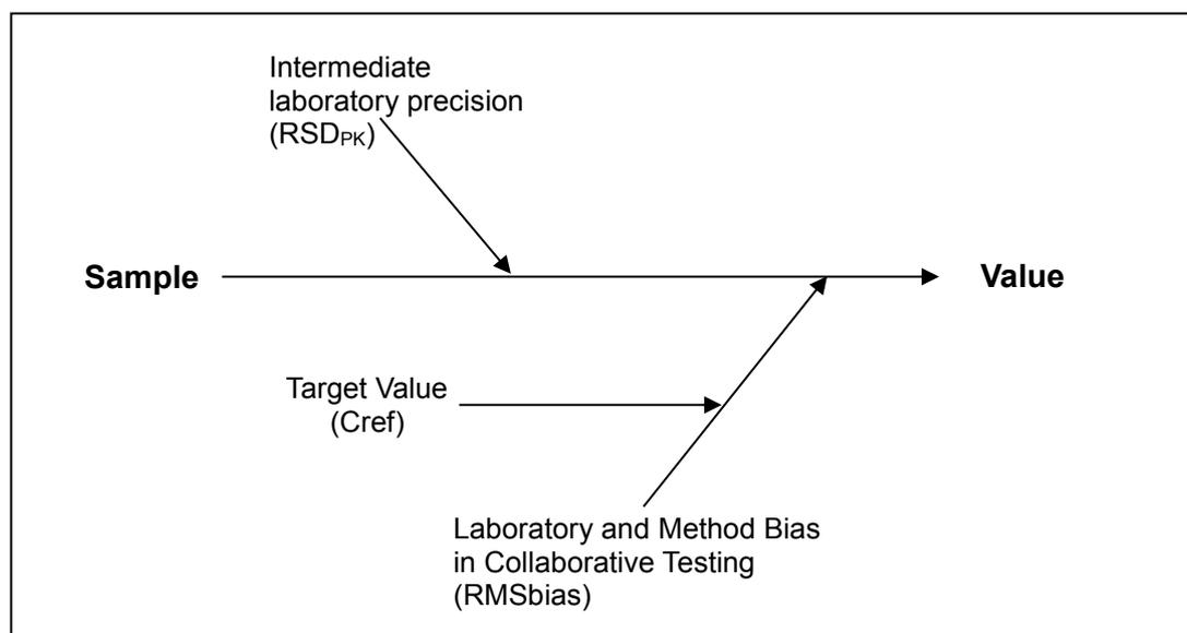
**Fig. 2: Cause-effect diagram for estimation of measurement uncertainty by using the precision and accuracy obtained from collaborative testing results and repeatedly measured control material (Nordtest Technical Report)**
